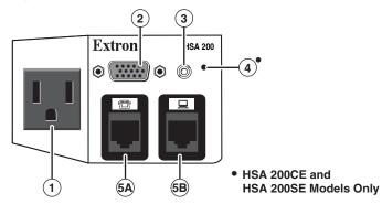
Figure 2-12 — HSA 200 front panel connectors
